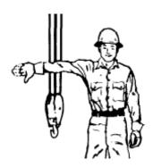
RAISE THE BOOM & LOWER THE LOAD: With arm extended, thumb pointing up, flex fingers in and out as long as load movement is desired.
