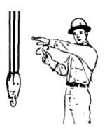
MOVE SLOWLY: Use one hand to give any motion signal and place other hand motionless in front of hand giving the motion signal.
