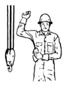
TRAVEL (One track): Lock the track on side indicated by raised fist. Travel opposite track in direction indicated by circular motion of other fist, rotated vertically in front of the body (Land cranes only)
