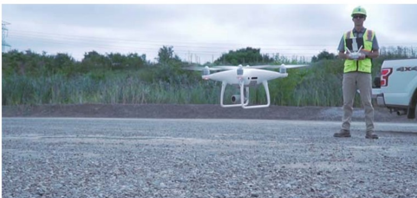
Figure 2. Flying a drone to capture aerial imagery for stockpile volume reports.
