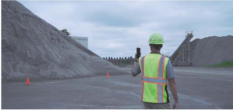
Figure 1. Measuring a stockpile using the Stockpile Reports Apple iPhone app.
